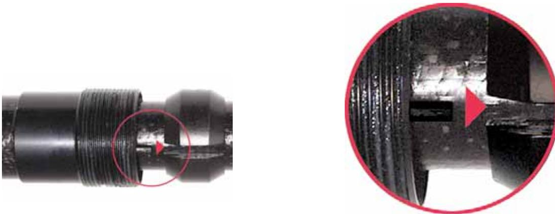
If a user opens the hand nut more than 5 turns then the pin can come out of its location in the ring. Then when the screwlock is retightened the pin may move away from its slot and will be bent or broken by the compression ring, which will be also be scored.
